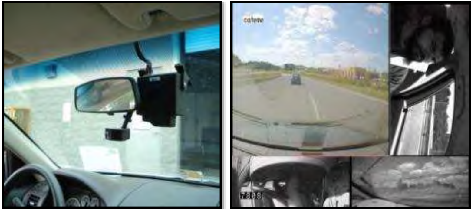
Figure 3.4. Head unit placement and camera views (source: FHWA, 2015, slide 15).
